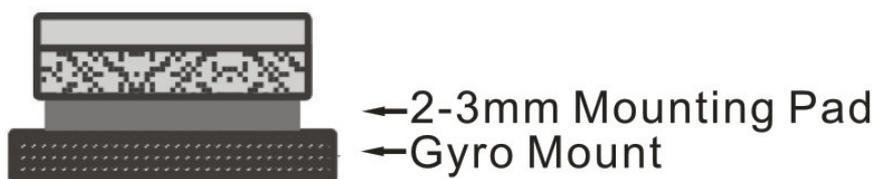
Mounting on a large or a High vibration helicopters: use a 2-3mm foam pad on each side of the damping shield plate.
